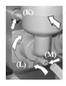
It is important to clean some of the machine parts regularly. This is important for the functioning of the machine, for the quality of the drinks and to fulfil the requirements for cleanliness. Maintenance work must be done with the power switched off. Cleaning must be done every week. Sometimes even more often depending on how often the machine is used. Neutral detergents must be used (avoid detergents that may harm colour or plastic). Never clean the machine by spraying water directly at it.
