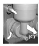
7. Fit the fixing plate by turning the selector clockwise. Check all seals!
