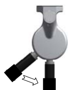
CORRECT POSITION OF THE PORTA-FILTER IN THE GROUP
