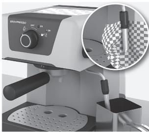
**4. Place a bowl under the steam nozzle** and turn the steam controller anti-clockwise for a few seconds, to remove hot water/milk from the steam nozzle. Turn the selector dial to the **OFF** position. Let the steam pipe cool down, then clean it with a cloth.
