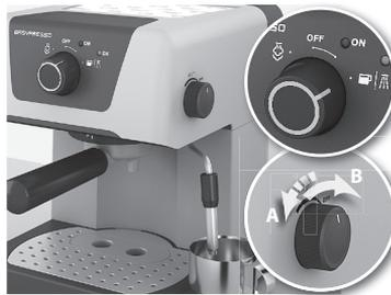
**5. For hot water**, place a cup under the steam nozzle, turn the selector dial to the ☕ position and the steam controller anti-clockwise (**A**). Hot water comes out of the nozzle. To stop, turn back the selector dial to **OFF** position. Then, turn the steam controller clockwise (**B**).
