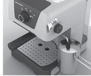
**3. Immerse the steam nozzle** in a heatproof container of milk/liquid, turn in a circular movement. (The nozzle should not touch the bottom of the container). Turn the steam controller anti-clockwise. Keep the nozzle in the container until you reach a desired amount of froth.
