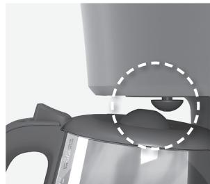
**5. If the jug is removed**, the filter valve prevents coffee from dripping onto the warming plate. (**While preparing coffee, the jug must not be removed for longer than 30 seconds or the filter will overflow.**)
