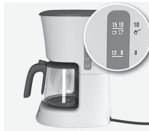
**2. Making coffee:** open the lid and fill the water tank with fresh cold water up to the desired level. There is a fresh water gauge for 2–10 big cups / 4–15 small cups in the water tank and on the coffee jug. (**The machine must not be used with empty tank!**)
