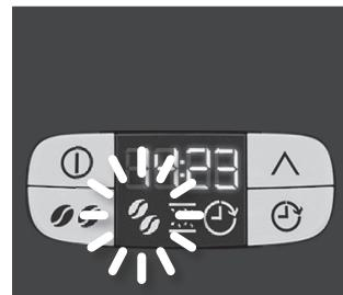
**9. The Aroma Selector** extends the brewing time to maximize the flavour extraction and get a stronger coffee for a small number of cups (normally less than 6). Press the Aroma button, the aroma icon will turn on.
