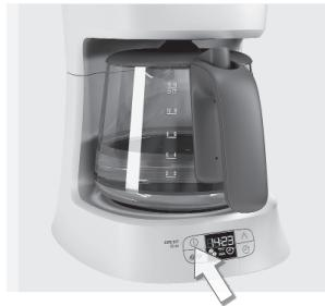
**4. Place the coffee jug with its lid** onto the warming plate. Allow the decalcifier to take effect for about 15 minutes, then switch the machine on. Switch it off when the solution has finished flowing through. If necessary repeat the decalcifying process.
