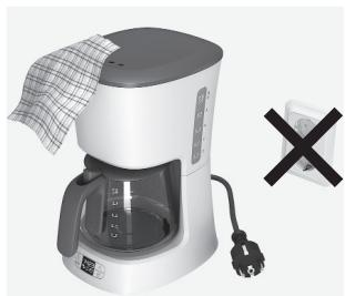
**1. Turn the machine off and unplug the power cord.** Wipe all outer surfaces with a damp cloth. Coffee jug and jug lid are dishwasher proof. **Never use caustic or abrasive cleaners, and never immerse the machine in liquid!**
