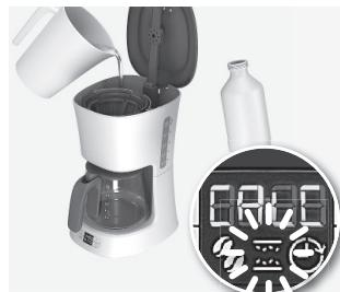
**3. Decalcifying.** After 150 cycles the text "CALC" appears on the display to indicate decalcifying is recommended. Fill the tank with water and decalcifier according to product instructions, then follow steps 4 and 5.
