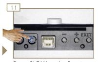
Press CLEAN on the Spectra S. The Spectra S starts the syrup priming.
