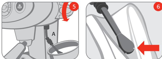
Immerse the steam arm in the milk **5**, turn the steam knob counterclockwise and wait for the milk to froth
