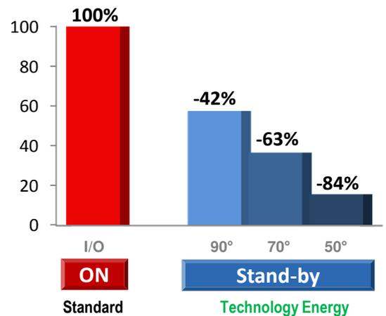
The **Energy Technology** is a significant saving of electricity. The electronic control of the boiler temperature drastically lowers the electricity consumption during standby moments of the machine.
