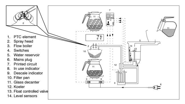
The coffee maker is equipped with a flow through heater system. This contains a water reservoir (5), a flow through heater (3), a sprayhead (2) from which the water flows into the filterpan (10), with in between a heat exchanger (12). The entire system is controlled by a printed circuit (7).
