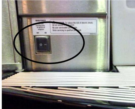
1. Press the power switch to the ON position to start the machine.
