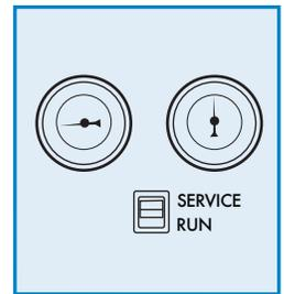
**14.** Push the service switch to the "Run" position. Secure cleaning materials and close all doors. The milk clean process is now complete.
