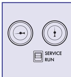
**10.** Push the service switch to the "Run" position. Secure cleaning materials and close all doors. The brew clean process is now complete.
