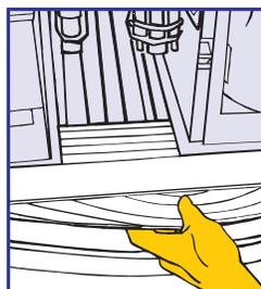
**8.** When the brew clean process is finished, open both front doors of the machine to clean the drain tray and grate. Remove and empty grounds bin.
