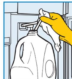
**13.** Using a clean cloth, re-insert milk pick-up tube into the milk container, and place milk container in the refrigeration unit.
