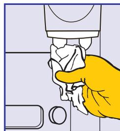
**9.** Wash delivery nozzles with hot, soapy water, and clean with sanitizer\*.
