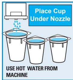
**6.** When **PLACE CUP UNDER NOZZLE** is displayed, place the first cleaning cup under the nozzle and press the **CLEAN** button. The cup will be filled with hot water. Repeat this process with the other two cups. The machine will beep after each cup is filled.
