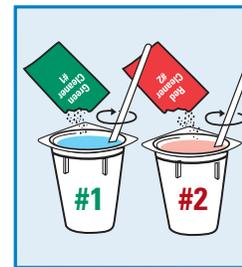
**8.** Slowly pour **Cleaner #1** into the first cup, and mix the cleaner and water thoroughly to ensure that the cleaning powder is completely dissolved. Repeat this process with **Cleaner #2** and the second cup of hot water.
