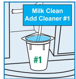
**9.** When the message **MILK CLEAN ADD CLEANER #1** is displayed, place the cup with **Cleaner #1** on the drain grate and place the milk pick-up tube in the cup, and press the **CLEAN** button.
