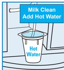
**11.** When the message **MILK CLEAN ADD HOT WATER** is displayed, place the cup with hot water on the drain grate and place the milk pick-up tube in the cup, and press the **CLEAN** button.
