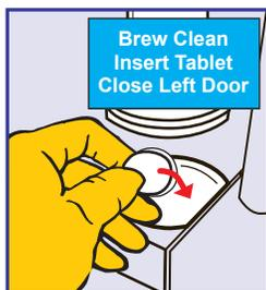
**7.** When **INSERT TABLET** is displayed, open left door and place one cleaning tablet in the grounds chute. **DO NOT** mistakenly place the tablet in the grounds chute. Close left door to begin the brew clean process.
