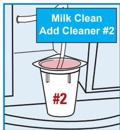
**10.** When the message **MILK CLEAN ADD CLEANER #2** is displayed, place the cup with **Cleaner #2** on the drain grate and place the milk pick-up tube in the cup, and press the **CLEAN** button.
