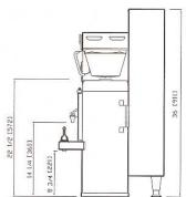
Water Requirements: 20-75 psig, 0.5 gpm flow rate. Water inlet is 3/8 Male Flare Tank Capacity: 3.7 gallons
