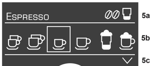
The status line **5a** in the display **5** shows the name of the type of drink, along with the strength setting, e.g.  $\emptyset\emptyset$  and per-cup quantity, e.g. . The selection line **5b** shows symbols for drink selection.
