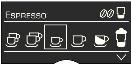
The status line **5a** in the display **5** shows the name of the type of drink, along with the strength setting, e.g. **00** and per-cup quantity, e.g. **□**. The selection line **5b** shows symbols for drink selection.
