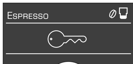
To deactivate the child-proof lock, hold down the °C button 3 for at least 3 seconds. The key disappears from the display 5.
