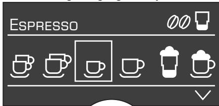
The status line **5a** in the display **5** shows the name of the type of drink, along with the strength setting, e.g.  $\textcircled{0}$  and per-cup quantity, e.g.  $\square$ . The selection line **5b** shows symbols for drink selection.
